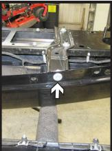
6. Pull back rubber piece. Using a T40 Torx, remove the three (3) bolts from the bumper. There are two (2) on the top and one (1) on the bottom. Do this on both sides of the bumper.
