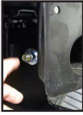
18. Place spacer plate onto 1/2" carriage bolt. Insert bolt and plate through access hole in the front of the vehicle frame. Install bolt and plate into side hole in baseplate and attach 1/2" flange whiz nut. Hand tighten. Do this on both sides of the vehicle.
