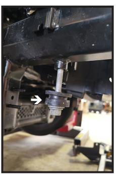
13. **Trucks with Tow Hooks:** Remove rubber grommet from back tow hook bolt and reinstall the existing tow hook bolt and hardware. Do this on both sides of the vehicle.
