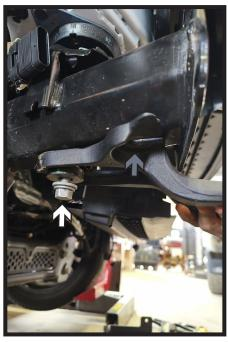
12. **Trucks with Tow Hooks:** Using an 18MM socket remove the front bolt (gray), and then using a 21MM socket remove the back bolt (white) attaching the tow hook to the frame. Do this on both sides of the vehicle. The tow hooks will not be reinstalled.
