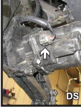
10. Using a 13MM socket, remove the two (2) nuts from the automatic valence. Do this on both sides of the vehicle. Unplug the electrical connection on the driver side and remove valence and set aside to be reinstalled later.
